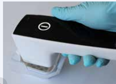
2 Mount the spacer to the device
